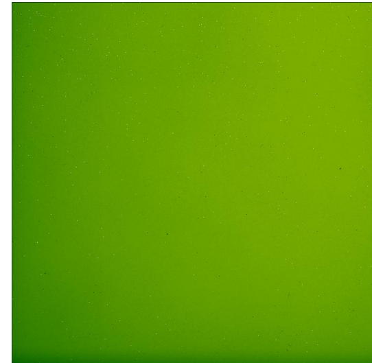
Correlated Double Sample (2 nd – 1 st read) Removes all offset artifacts
